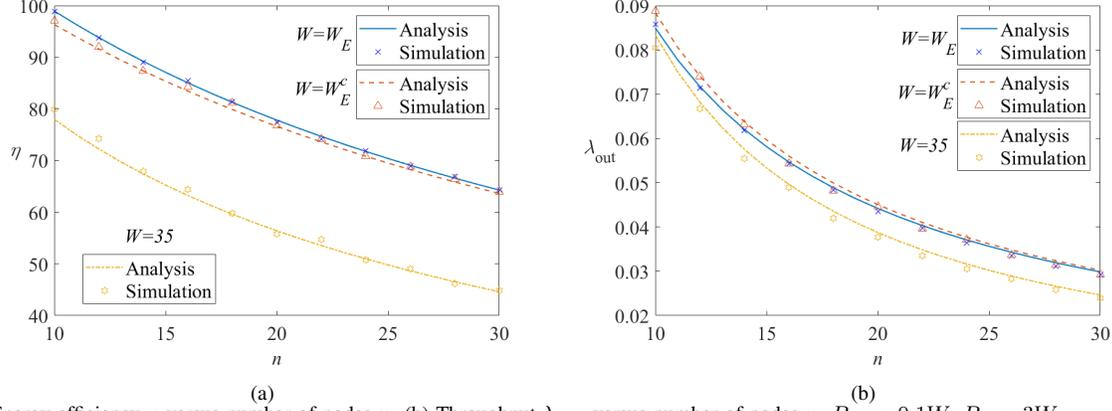
Fig. 5. (a) Energy efficiency  $\eta$  versus number of nodes  $n$ . (b) Throughput  $\lambda_{out}$  versus number of nodes  $n$ .  $P_W = 0.1W$ ,  $P_T = 3W$ ,  $\tau_F = 2.37 \times 10^{-3}$ s,  $\tau_T = 2.45 \times 10^{-3}$ s,  $K = 6$ ,  $m = 2$ ,  $\lambda_0 = 90\% \lambda_{max}$ .
