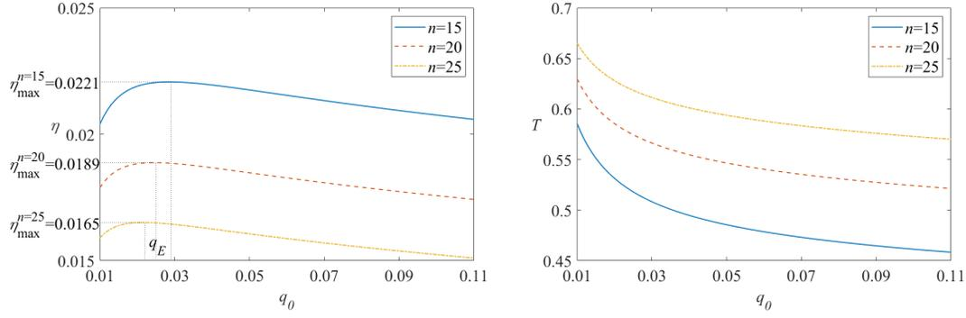
Fig. 3. (a) Energy efficiency of each node  $\eta$  versus the initial transmission probability  $q_0$ . (b) Lasting time  $T$  versus the initial transmission probability  $q_0$ .  $E = 1$ ,  $P_W = 1$ ,  $P_T = 20$ ,  $a = 0.1$ ,  $x = 5$ ,  $K = 6$ ,  $Q(i) = 2^{-i}$ .
